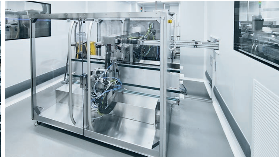
Depending on the format, the blisters are not directly forwarded to the cartoner but automatically buffered in trays and cartonized at a later point in time.
