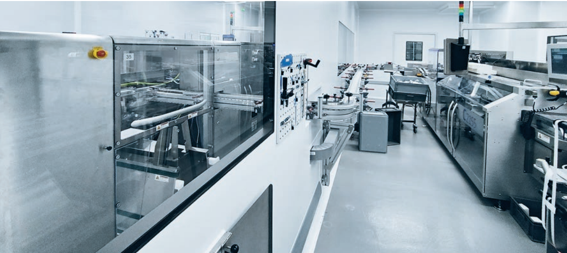
The blister machine and cartoner are physically separated at Synthon. The sealed blisters reach the cartoner via a conveyor belt.
