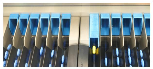
Uhlmann is presenting its innovative single tablet reject function for the pharmaceuticals packaging line IBC 150 at Pack Expo in Chicago. This optional module checks the tablets already in the tablet counter and identifies any damaged or incorrect products and foreign particles. These are rejected whilst maintaining a high production speed.
