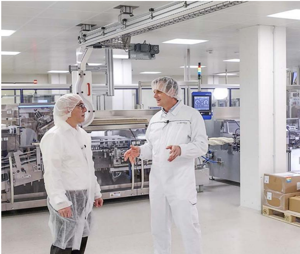
Figure 2: Photo cartoner for blisters and bottles
