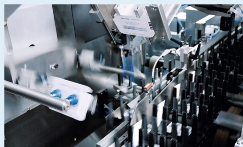
Rotary carton pick-up with suction cups
