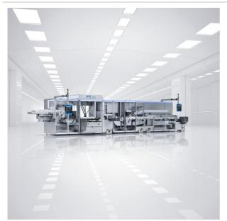
The PTC 200 Parenteral Tray Center is characterized by its extremely high flexibility in terms of packaging material and product shapes: It processes sustainable carton packaging, cardboard and plastic trays. (Source: Uhlmann)
